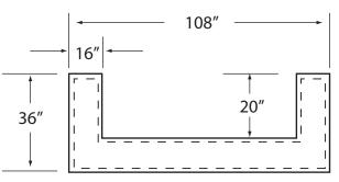
27 foot Warm White installation above and above left includes 2 - CFX2V2-60-WW (97.2 watts for 27 feet) and 1 - LED-TR-150-24 (65% of capacity) or 1 - LED-DR100-24 (97% of capacity).
