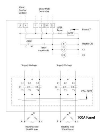
Smplified three phase connected heating cables
