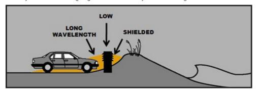
**Keep it LOW** - mount the fixture as low as possible to minimize light trespass, and use the lowest amount of light needed for the task. **Keep it SHIELDED** - fully shield the light so bulbs and/or glowing lenses are not visible to minimize light trespass.
