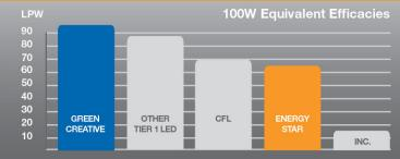
At 97 LPW, this lamp's efficacy is 10% higher than the Tier 1 LED A21 100W replacement industry average and exceeds new ENERGY STAR requirements by upwards of 50%. This energysaving performance makes this lamp a smart retrofit choice for incandescent and CFL bulbs.
