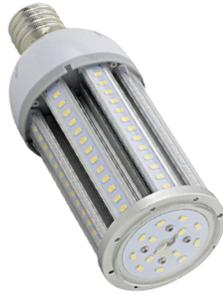
The ProLED® HID Retrofit Series lamps are an easy to install LED solution for post top and high bay fixtures. ProLED HID Retrofit lamps offer an energy-efficient alternative to traditional High Pressure Sodium and Metal Halide lamps. The 36W ProLED HID Retrofit lamps can be used in enclosed luminaires. The series is available with 82 CRI and 5000K color temperature.
