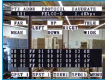
PTZ protocol analyzer can be used in-line to troubleshoot keyboard controllers and cameras
