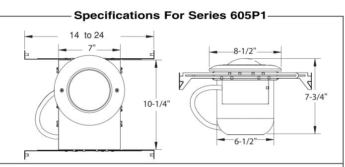
**GENERAL:** The contractor will furnish and install 6 volt emergency lighting units, as indicated on all plans. Units shall be designed for recessed ceiling installation. Input power shall be 120/277 volt 60 Hz.
