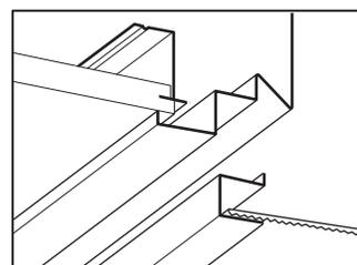
Exclusive LIGHT-LOCK™ design for tight light fit of door to housing. Diffuser inserted without the use of tools
