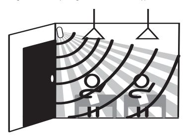
The versatile OSW12-M Occupancy Sensor can be mounted on the wall to provide full room coverage when low-hanging lights or other obstacles are present. Infrared and ultrasonic signals are used for maximum reliability.
