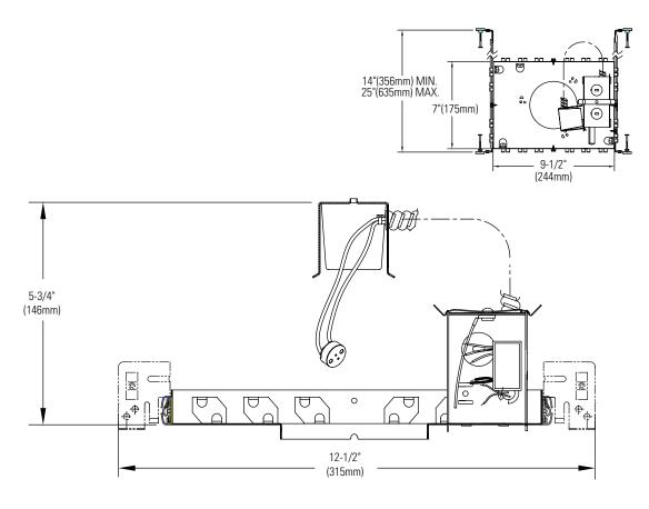
Complete fixture consists of Reflector Trim & Frame-In Kit. Select each separately
