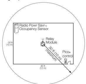
In larger spaces such as conference rooms (where the longest room dimension is greater than 21 ft/6 m), place the module in the center of the room to ensure RF coverage.
