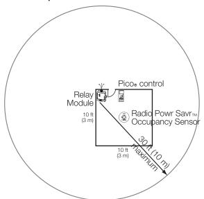
In smaller spaces such as private offices (where the longest room dimension is less than 21 ft/6 m), place the module above the door to facilitate locating it after installation.
