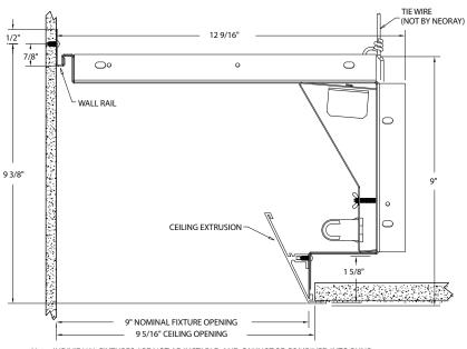
Note: INDIVIDUAL FIXTURES ARE NOT ADJUSTABLE, AND CANNOT BE COMBINED INTO RUNS. If adjustability is required, use 790S continuous fixture.
