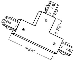
To connect three sections in a T configuration. Field adjustable for right or left polarity. Can be used as a power feed.
