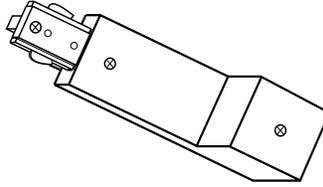
Accepts standard 1/2" trade-size conduit fitting. Use with surface conduit feed.
