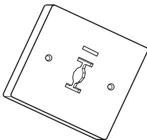
For use with line voltage fixtures, NTH series. Mount to outlet box.
