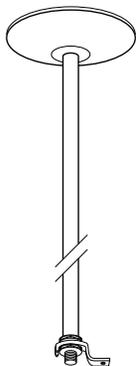
Stems are 5/16" hollow rod with right hand screw threading. Kit includes stem, canopy, cover for back side of track and hardware. Minimum 2 pendants per track up to 4' track section or 1 per end then every 4' thereafter.
