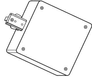
To start a run on a T-Bar type ceiling. Mounting hardware included.
