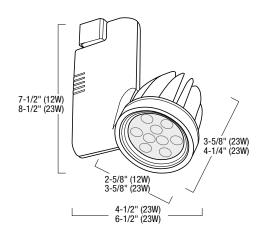
Width: 4-1/2" (12W) / 6-1/2" (23W) Length: 3-5/8" (12W) / 4-1/4" (23W) Diameter: 2-5/8" (12W) / 3-5/8" (23W) Max. Extension: 7-1/2" (12W) / 8-1/2" (23W)
