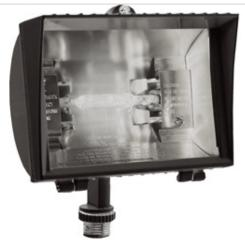
The Mini Curve. High quality die cast flood with rounded back and integral glare shield. Tempered glass lens. Gold plated socket contacts and 250°C Teflon coated wires for extended lamp life. 150 Watt double ended 130 volt Quartz halogen lamp supplied.
