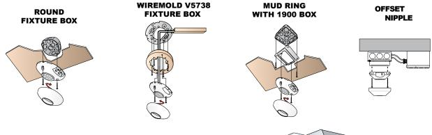
The fixture (CMRB) sensor enclosure provides an extended chase nipple that facilitates mounting to a half-inch knockout hole on the side of a fixture.
