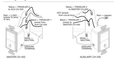
For single pole applications, cap off the yellow wire. Up to four multi-location sensors may be connected together. For details on connecting RH-253s for multi-location control, see the RH-253 cut sheet.
