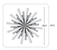
Coverage shown is maximum and represents half-step walking motion. Under ideal conditions, coverage for half-step walking motion can reach up to 1000 sq ft.
