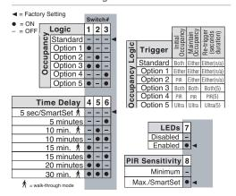
The technology control (occupancy logic) options are adjustable by user. The standard setting (recommended for most applications) is both technologies to trigger on, either to hold on.
