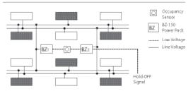
The occupancy sensor connected to each BZ-150 keeps all lights on when the space is occupied. When the load shed command is given (by utility meter, BMS, etc.), lights connected to BZ $_2$  are held off. Remaining lights (connected to BZ $_1$ ) are still controlled by occupancy sensor.
