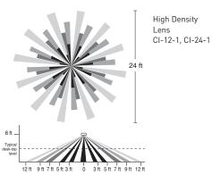
Coverage shown is maximum and represents coverage for half-step walking motion. Under ideal conditions, with no barriers or obstacles, coverage for half-step walking motion can reach up to 1200 ft² using the Extended Range lens and up to 500 ft² using the High Density lens. For typical desktop level of activity, coverage can reach up to 300 ft² using the High Density lens.
