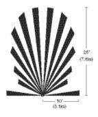
The WN-100 has a coverage range of 180 degrees and a maximum coverage area of 300 sq ft (28 m²). To maintain its coverage capacity and optimally detect motion, the WN-100 must have a clear and unobstructed view of occupants.
